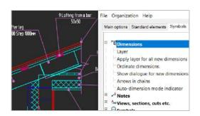
The Construction module supports drawings with many views at different scales. With just two clicks, you can adjust the scale of drawings, both for specific objects and for entire drawings. The symbol scale adjusts the sizes of text, dimensions, and line types automatically in model space and in layouts using viewports.
