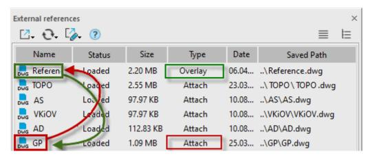
In previous versions of nanoCAD, it was impossible to create or edit an existing system of cyclic references - once such a reference was deleted, it either could not be reconnected (there was an error **Possible circular reference to current drawing**), or it was necessary to break the links for each file.
