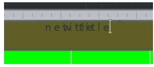
The bug when while editing an existing text in a DWG table cell (DTABLE command) it was impossible to delete this text - after editing the cell, the text was displayed again.
