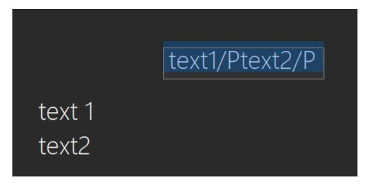
The error in the display order of raster images after aligning the underlying raster with the ALIGN command has been fixed. After applying the command to a raster image, it was displayed above other images, until the viewport was updated (REGEN).
