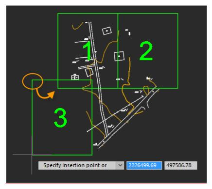
For cycle change of the anchor point, just press the **Spacebar** key or select the **Anchor point** keyword. Anchor point can be set to any vertex of the frame:
