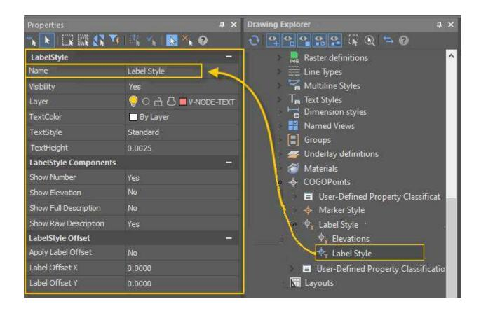
Editing properties of marker styles is started by double clicking on the required marker style in the **Drawing Explorer**. The parameters are set in the **Properties** bar.
