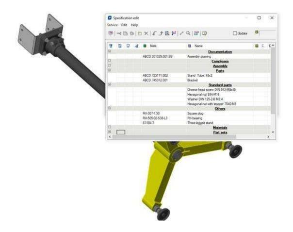
In views of 3D model of an assembly, you can place numbered leaders of specification positions. Specification leaders position numbers are synchronized with the specification editor, and specification elements can be renumbered.
