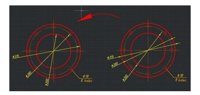
The error in constructing a radius dimension when creating a connection, when only an arrow was displayed without a dimension line.
